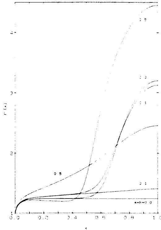
Fig. 17. Stable (—) and unstable (---) cylinder profiles for three different slopes in initial thickness and radius variations with R_p = 0.571 , S = 10 and \lambda_{10} = 1.05 .
